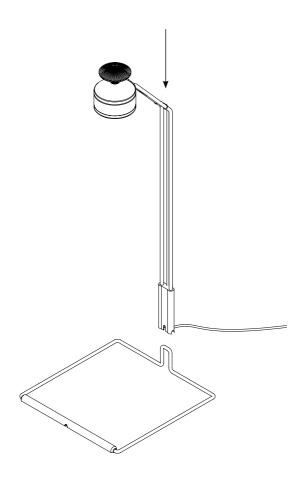
Insert the set screw into the back of the connecting piece and screw it firmly in place, using the supplied tool.
