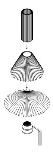
Once the shade is in place, gently adjust the pleats at the top so they are evenly spread out, as shown below. Once the shade is as illustrated, the top screw can be fully tightened.
