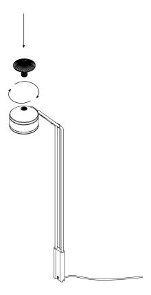
Slide the stem onto the base frame, as shown below.
